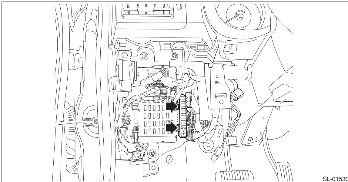
5) Remove the relay & fuse box.
