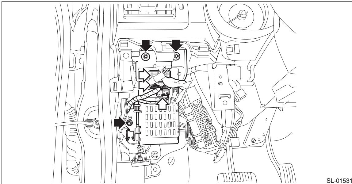
6) Remove IG relay 1 (push button start) (A) from the relay holder.
